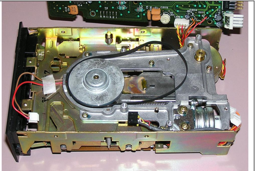
Once the cables are replaced, be careful when placing the main board back onto the chassis. Ensure line up the drive LED and slide it into the plastic slot on the reverse of the drive front plate as shown, or it may get bent or worse break off.
