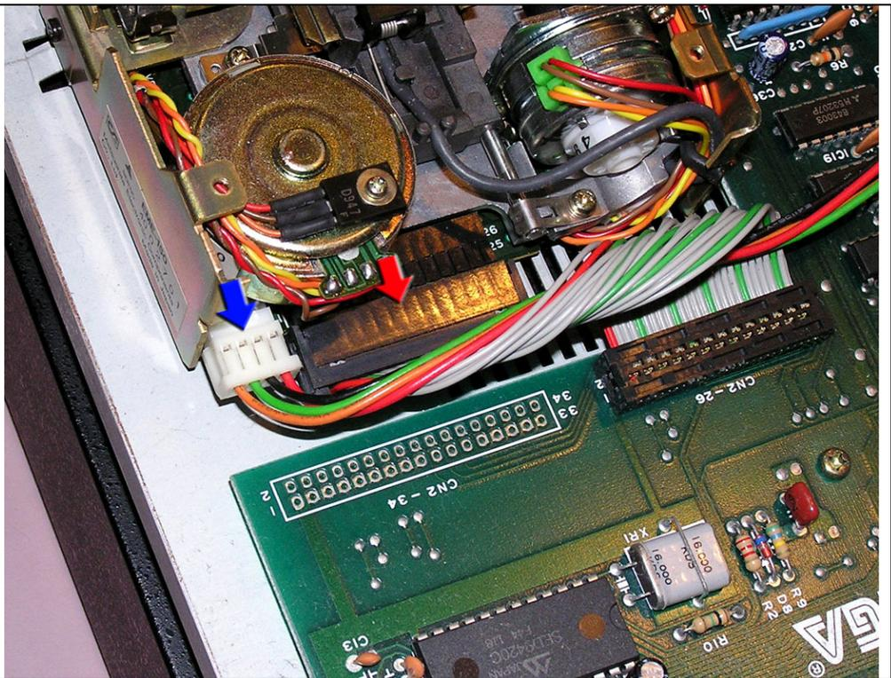
Turn the SF-7000 upside down and remove the 3 screws securing the 3" Drive to the SF-7000 casing.
