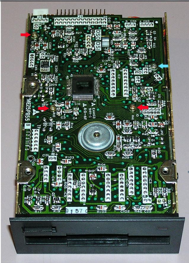
Looking from the back of the drive, remove the two small cables going to the main board from the Stepper Motor and Head.
