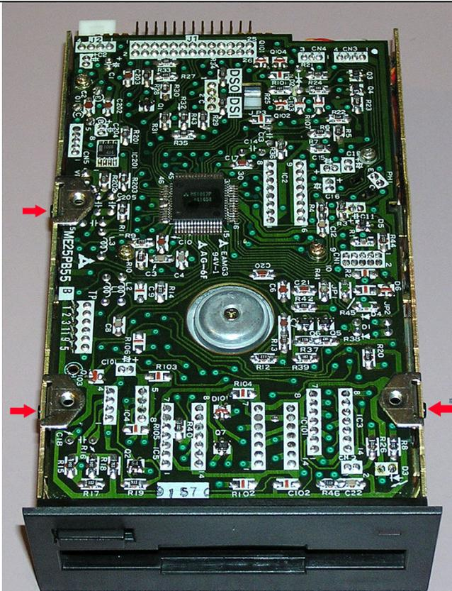
Locate the 4 screws holding the Drive's main board down, and remove.
