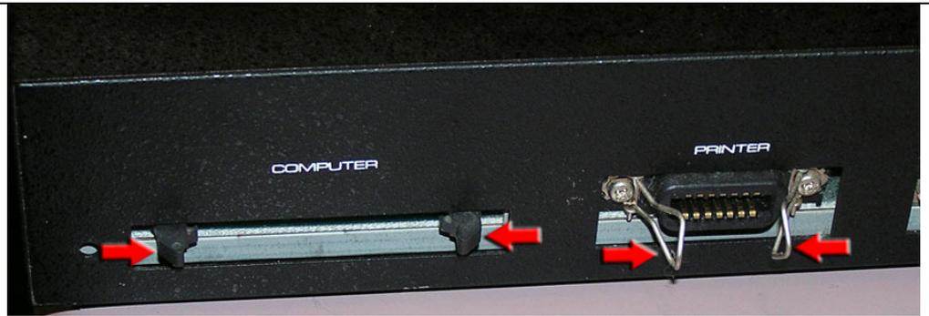
Then screw in the two case screws on the back of the SF-7000.
