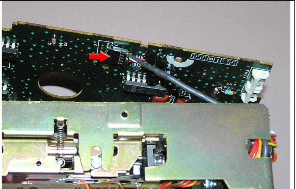
We can leave the remaining cables connected to the main board. As we can see the drive belt now. Remove the drive belt from the large wheel and then the small wheel, and place aside.
