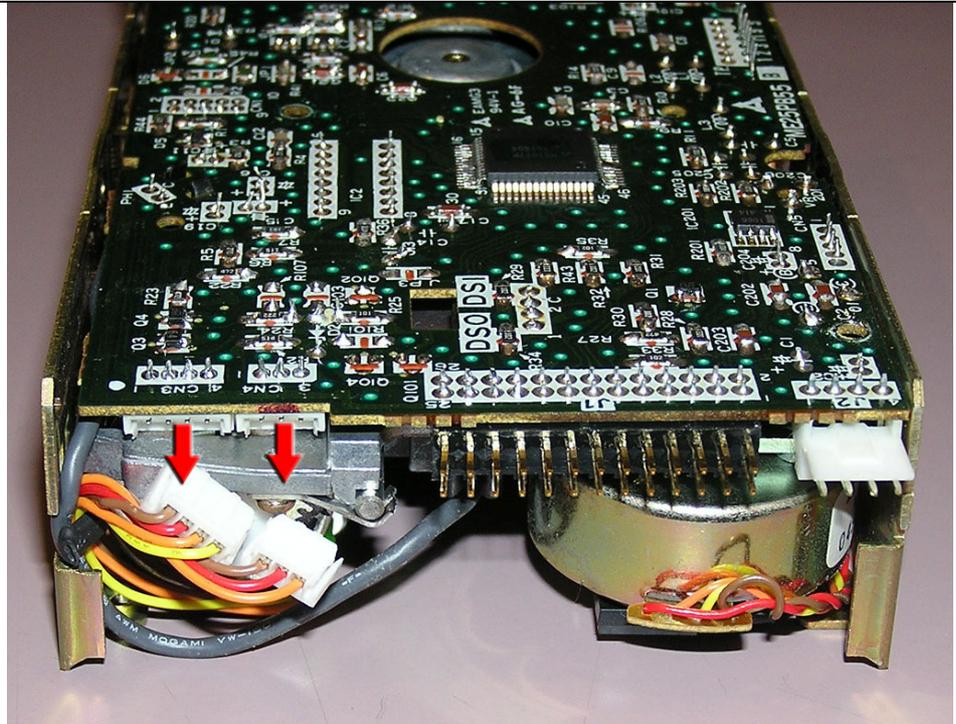
Turn the drive around so you are looking at the front of the drive, remove the small cable on the underside of the main board.
