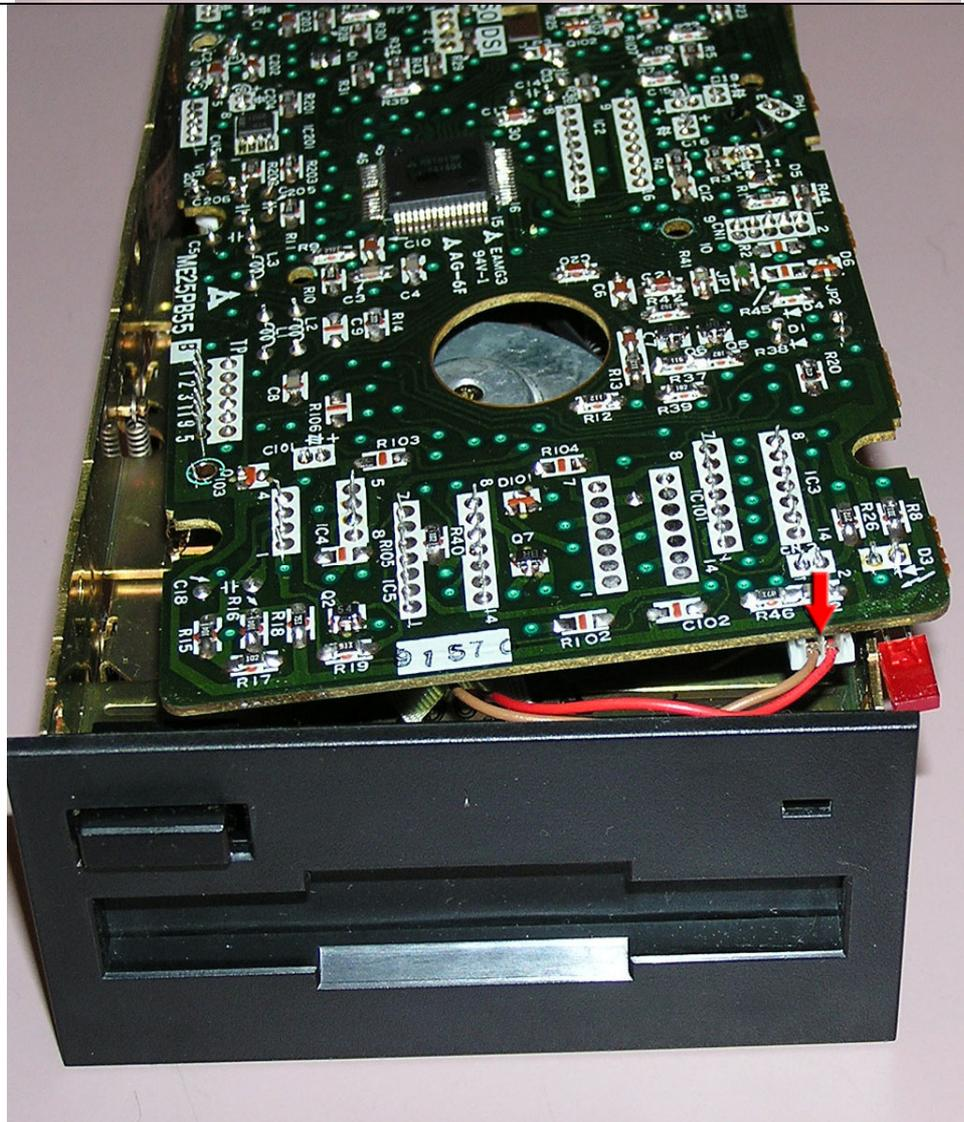
Now turn the drive around to the side (side closest to the LED) and remove the small cable on the underside of the main board.
