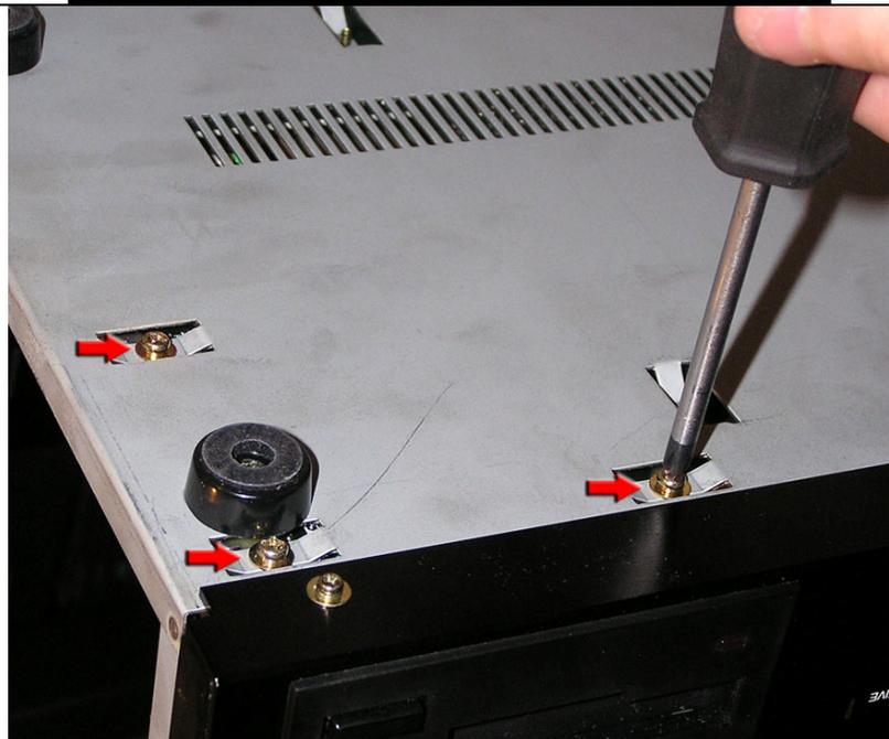
Then slide the top of the SF-7000 case back along from back to front. Watch out for the Power cable that can get in the way, and also ensure that the Computer and Printer latches/clips are out of the way by pushing them in towards each other.
